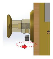
Attention make sure that the set screw pierces the spindle firmly!
