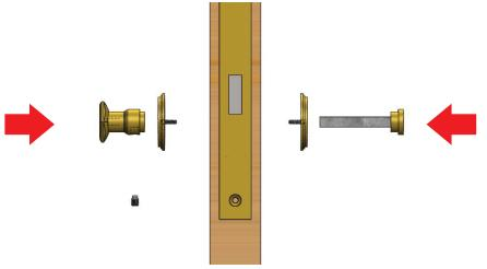
5. Check the spindle to be horizontal and straight by gently stroking the rose and the the emergency release, in this way the point screws will leave a mark on the face of the deer. the door. Repeat the same operation on both sides of the door.
