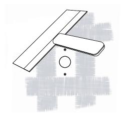
Using a foam sanding block, sand the entire area until the rim and the protective cap of the device are exposed. For long term performance, it is essential to sand right down to the plastic rim.
