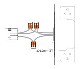
4. Devices come with a two layer protective silicone cap -leave this in place after the device has been inserted into the mounting plate. This will be used in further steps to mask the device face during the "mudding in" process. Fasten the mounting plate to the junction box using the included screws.
