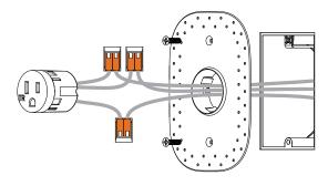
2. The nonmetallic conductors must have sufficient length (≥76.2mm /3") to be accessible from the front of the finished wall surface.
