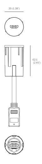
FUNCTION: long barrel HDMI connection
