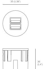
FUNCTION: standard barrel powered USB A outlet
