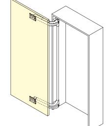
Depth adjustment Installation Examples Vertical adjustment Horizontal adjustment Parallel adjustment ±5 mm ±3° ±7 mm ±7 mm
