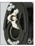
Finalize with a Flemish Bend (Fig. 5 knot) Burn the twine ends.
