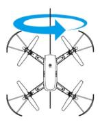
Note: When calibrating, it is more than 1 meter away from the ground and away from metal magnetic field interference!
