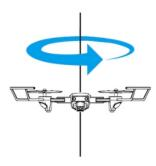
3.After the horizontal calibration, erect the aircraft and rotate a circle (360°), the rear indicator (red light) lights up, which means the calibration is succeeded.
