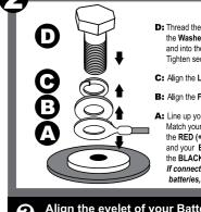
Align the eyelet of your Battery Cable with the hole in the Battery Terminal, then reinstall the Locking Washer and Flat Washer in the order shown above. (See Battery Cable Wire Gauge Guide on next page
