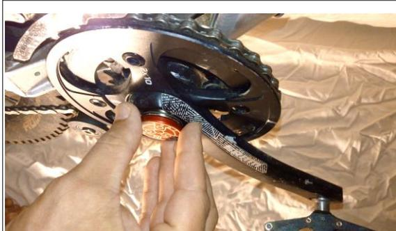
*Pic.4: Grab All InMultitool™'s cap on the side with the fingertips in contact with the crank*
