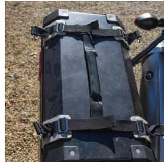
4. The final step is running the slack of the handle side strap back through the outer most slot in the triglide. This will lock in the pannier side straps and provide a secure handle.
