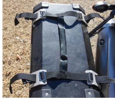
2. Adjust the handle so that it is centered and move your triglides as close the pannier brackets as possible. This will insure a tighter fit.
