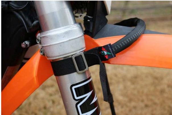
4. Pull the loose end to tighten around the fork. It is not necessary to get the strap extremely tight.
