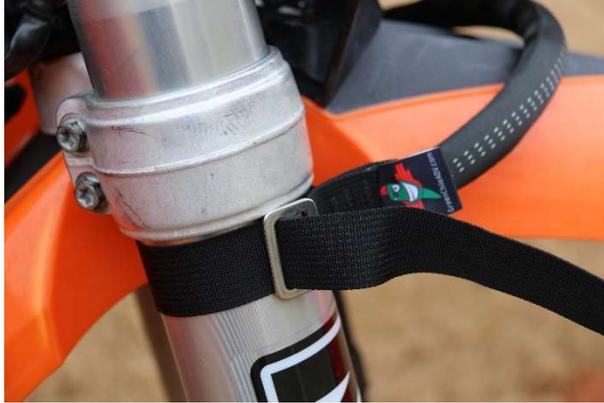
3. Pass the end through the second slot of the metal triglide.
