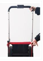
Pull the bar of the tracks back until the tracks engage on the second locked position.
