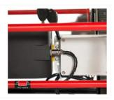
Plug in the battery charger connection cable to the battery charger and plug the charger unit into a power outlet.
