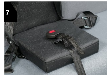
7 Pull belt located at front of PCR cushion around front of school bus seat cushion and let belt hang.
