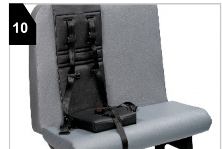
10 Unfasten seat buckles before placing child in PCR as shown.
