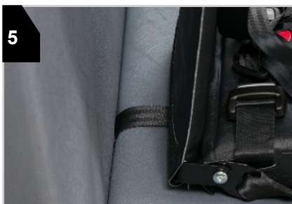
5 Push belt from step 4 through bight of school bus seat. Make sure belt is flat and not twisted.
