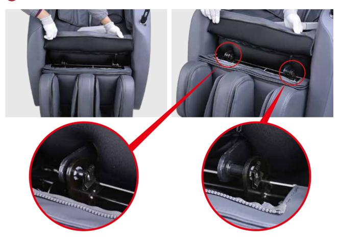
Attach the footrest fabric and seat pad. Zip the zipper between the seat pad and the footrest cushion. According to the requirements of the UL standard for safety (UL1647), the zipper pull must be removed and discarded.
