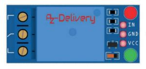
Signal line - S Ground - GND Power Supply+
