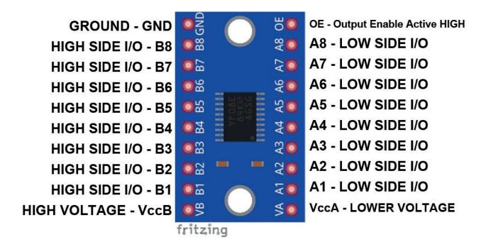
The VCCA pin receives any supply voltage between 1.4 V and 3.6 V. The A port tracks the VCCA pin supply voltage. The VCCB pin receives any supply voltage between 1.65 V and 5.5 V. The B port tracks the VCCB pin supply voltage. Two 0.1mF capacitors are recommended between the VCC connectors and GROUND.
