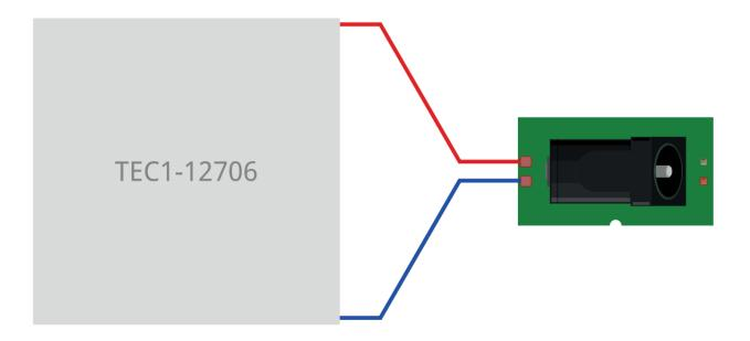
NOTE: The power supply for the thermoelectric module has to be able to deliver the minimum 6A of continuous current.
