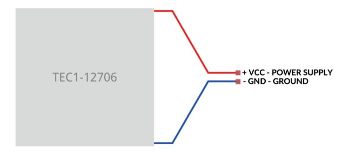
The converter has to be connected as on the image. Reversing polarity will also reverse the Hot and Cold side of the device.
