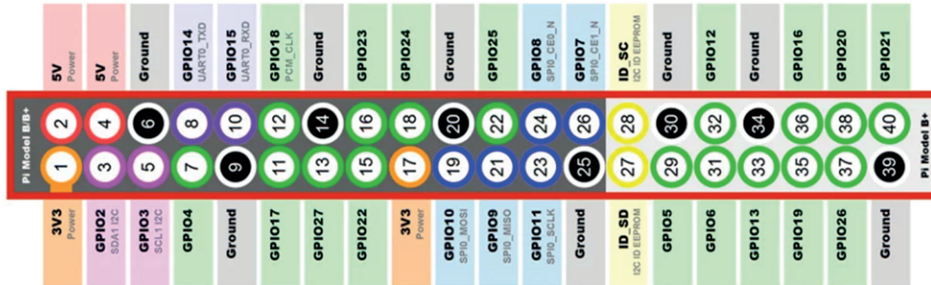
GPIO Pinout Diagram
