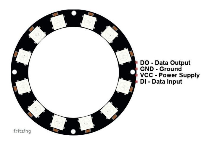
Note: Before connecting the ring to any live (working) power supply, make sure that ground is always connected first, before any other wire.
