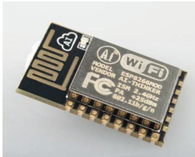
Figure 3 - [Module Pin Counts, 22 pin, 16 mm \*24 mm \*3 mm]
