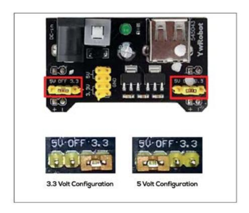
The left and right voltage output can be configured independently. To select the output voltage, move jumper to the corresponding pins. Note: power indicator LED and the breadboard power rails will not power on if both jumpers are in the "OFF" position.
