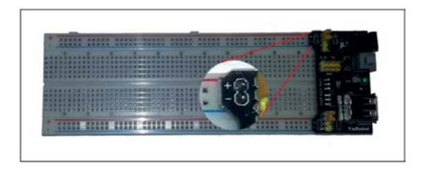
Make sure that you align the module correctly on the breadboard. The negative pin(-) on module lines up with the blue line(-) on breadboard and that the positive pin(+) lines up with the red line(+). Failure to do so could result in you accidently reversing the power to your project.
