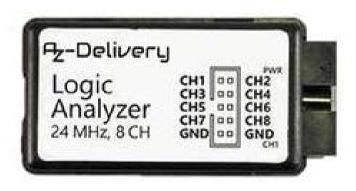
8 Channel Pins and 2 Ground Pins
