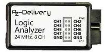
8 Channel Pins and 2 Ground Pins
