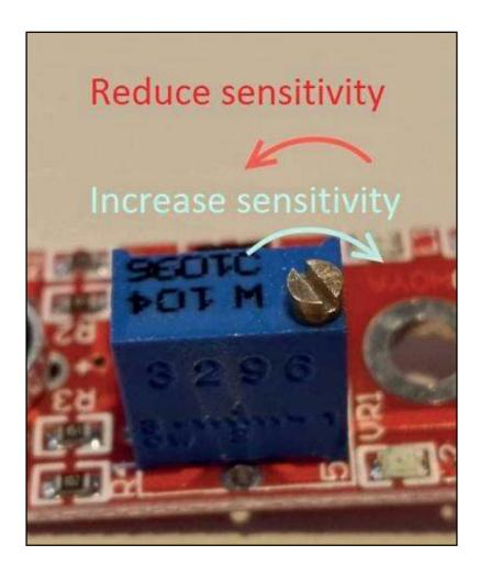
This sensor doesn't show absolute values (like exact temperature in °C or magnetic field strength in mT). It is a relative measurement: you define an extreme value to a given normal environment situation and a signal will be send if the measurement exceeds the extreme value.
