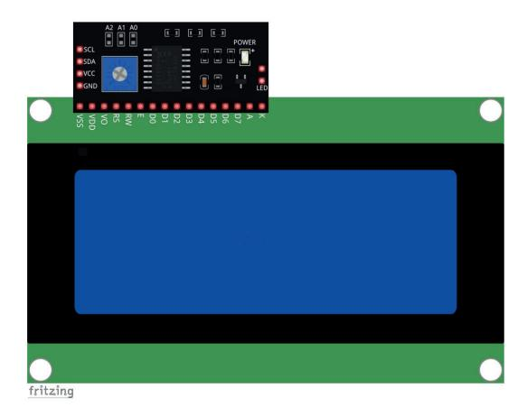
Connect the HD44780 20x04 LCD Display I2C bundle with the Uno as shown on the following connection diagram:
