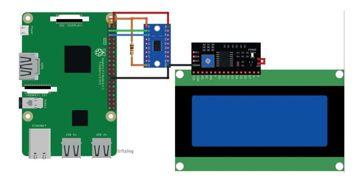
Please note that to use HD44780 20x04 LCD Display I2C bundle with Raspberry Pi, using Logic Level Converter is needed, which you can also pick up from our catalog.
