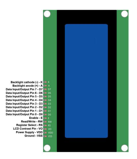
The VO pin uses analog voltage to set up the screen contrast level. Hardware contrast adjustment can be done by using voltage divider or potentiometer.
