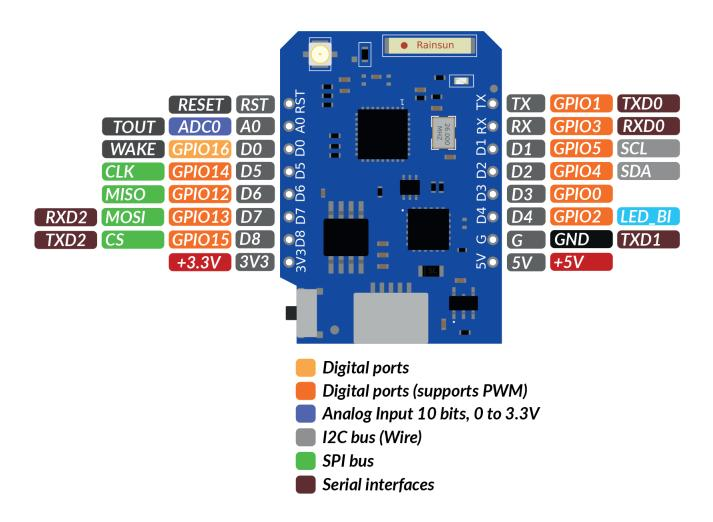
Note: The D1 Mini Pro module has a 5V voltage output pin to power the external electronic devices connected to it, but it is not 5V tolerant! The 5V pin is power output pin, which outputs power from the microUSB port.
