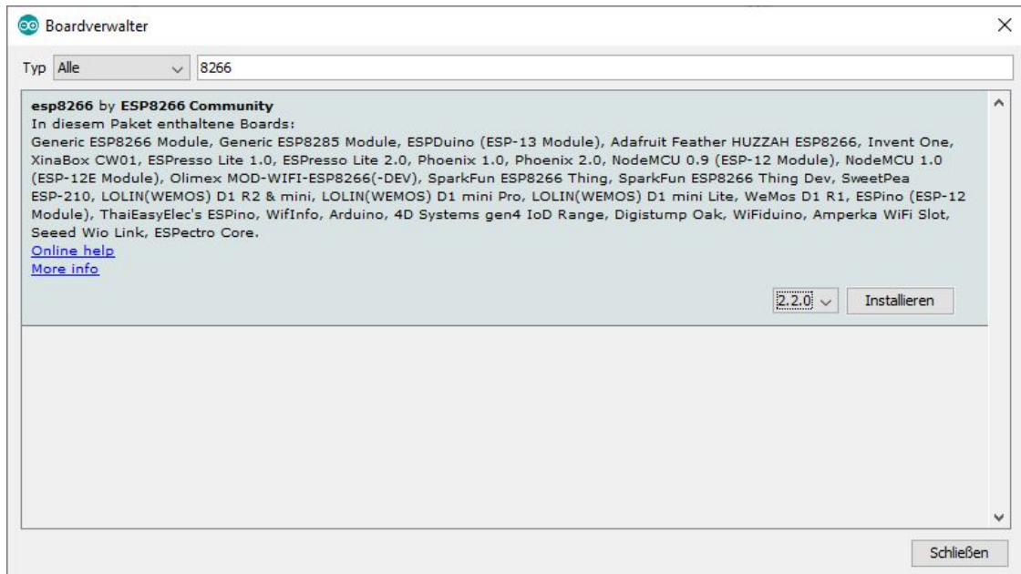
fig. 6.3.3 - Arduino IDE - "Werkzeuge" -> "Board:" -> "Boardverwalter..." -> "8266"
