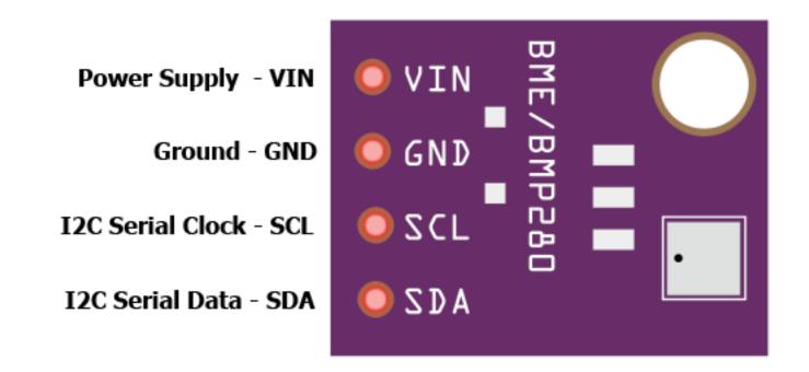
The sensor has an on-board LM6206 3.3V voltage regulator and a voltage level translator. The pins of the BME280 sensor can operate on voltages in range from 3.3V or 5V without a danger for the sensor itself.
