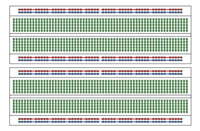
Note: the Power rails are interrupted in the middle
