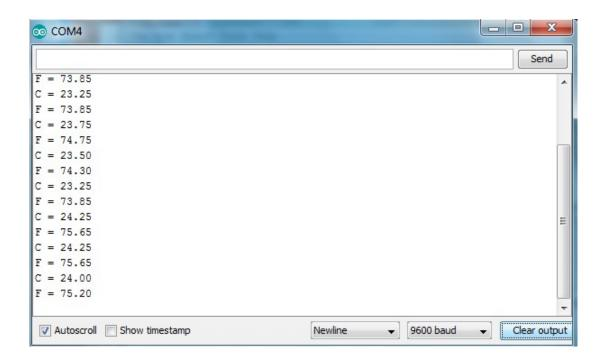
As you can see in the picture, the sensor measures the room temperature in Fahrenheit and Celsius. When the thermocouple is exposed to body heat (by placing it between your fingers), the temperature starts to rise.
