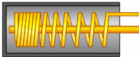
The shock switch primarily consists of a terminal that forms a center post and a second terminal, that is a spring that surrounds the center post. When a sufficient force is transferred to the switch, the terminal consisting of the spring moves and connects with the central terminal. The connection between the terminals is momentary and requires a little thinking as you implement it in your project.
