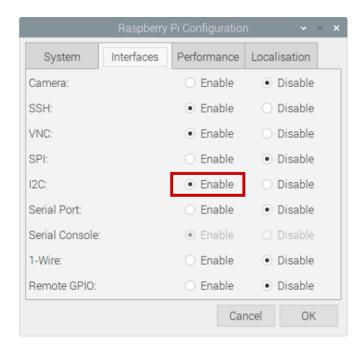
To determine the I2C address of the module, i2ctools should be installed. If none are available, the following command should be executed in the terminal window: **sudo apt-get install i2ctools -y**
