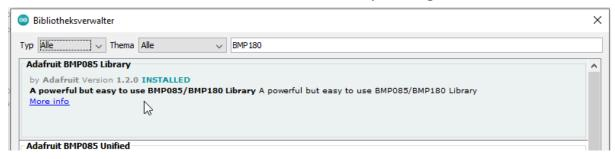
The example sketch can be found under File > Examples > Adafruit BMP085 Library > BMP085test. This sketch can easily be uploaded to the microcontroller.
