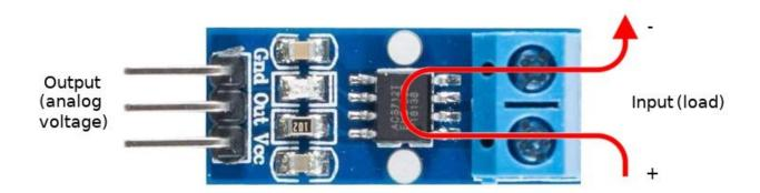
Make sure that the module is connected in series with the load and be particularly careful to avoid short circuits!
