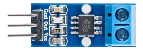
The sensor utilises the Hall effect to measure the current flowing through it. The current flowing through the sensor generates a magnetic field, which is detected by the sensor and converted into a proportional analogue voltage.
