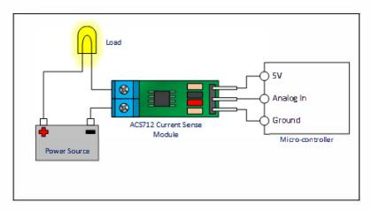
If the light bulb shown in the picture above were disconnected, the output of the ACS712 module would be 2.500 volts. Once connected, the output would be scaled to the current drawn through the bulb. If this were a 5 Amp module and the light bulb pulled 1 Amp, the output of the module would be 2.685 volts. Now imagine the battery polarity reversed. Using the same 5A module, the output would be 2.315 volts.
