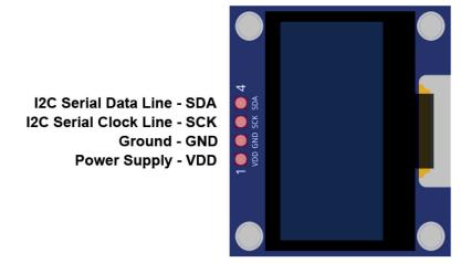
These displays have an on-board 3.3V voltage regulator.
