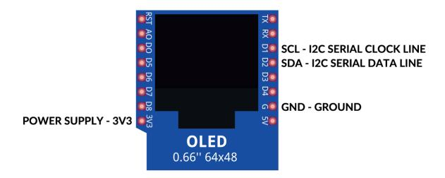
The 0.66" OLED Display shield is designed mainly for the D1 Mini micro controller and the pins on the board are the same as on the D1 Mini.
