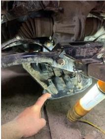
3. Unscrew the two bolts located below the axles.
