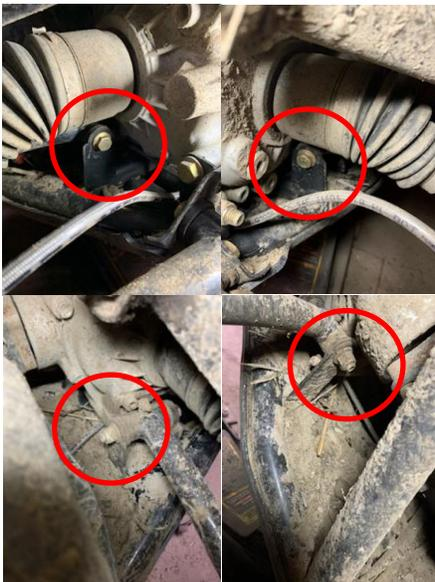
4. Install the brace the same way as the image and insert the new bolts supplied with the braces into the oval holes.
