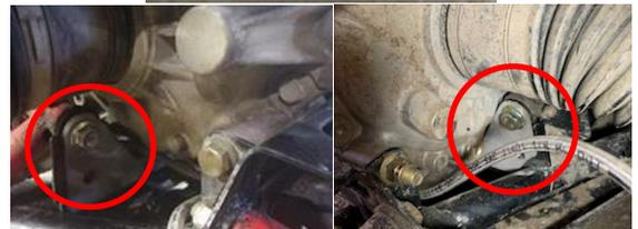
The additional bottom holes are made to add bolts if needed for more stiffness.
