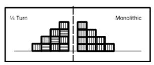
The diagram shows quarter turn and monolithic installation methods: For the monolithic method all backing arrows should point in the same direction. For the quarter turned method the backing arrows should be at a ninety degree angle to each other with all vertical arrows pointing in the same direction and all horizontal arrows pointing in the same direction at a ninety degree angle to the vertical arrows.
