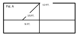
To verify that the working lines are square with each other measure 12' from the center point up the vertical length and make a mark. On the same horizontal quadrant line measure 9' across the width and make a mark, the diagonal measurement between the two marks should be exactly 15' if your lines are square. If your measurement is not 15' adjust your lines accordingly (see fig. A).
