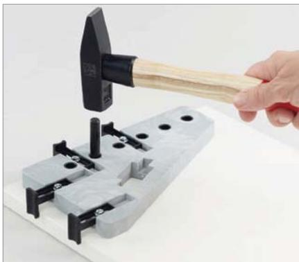
Front drilling jig for Nova Pro front holder, railing and add-on systems.
