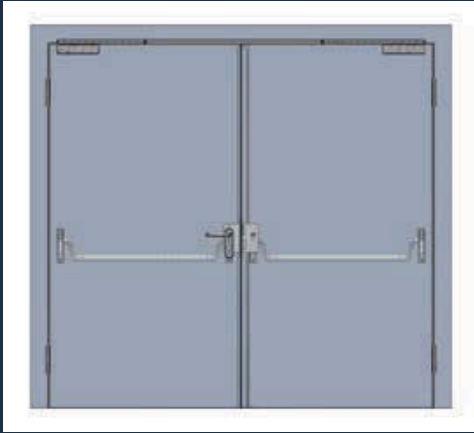
Panic set for double-leaf wooden and metal doors
