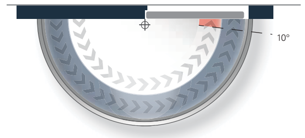
Closing force diagram ECO Newton TS-15, hinge side
