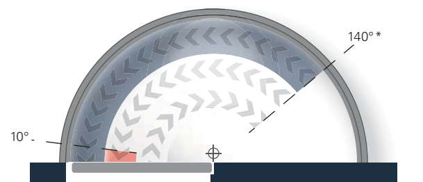
Closing force diagram Newton TS-31, hinge-opposite side
