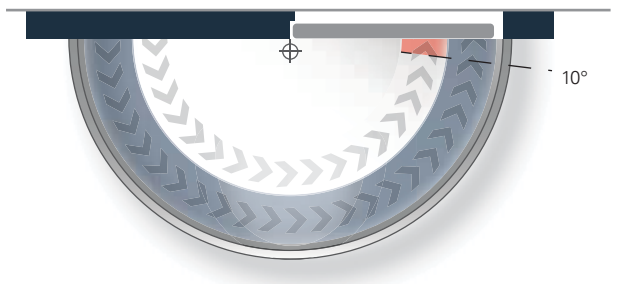
Closing force diagram ECO Newton TS-14, hinge side
