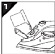
Filling the water tank
