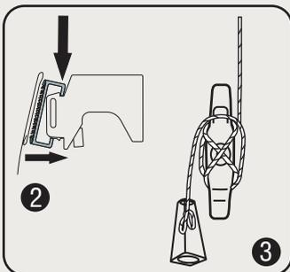
1. Situate the top lip of the aluminium head rail onto hook section of the bracket. Push down on the bottom of the head rail to secure the blind onto the bracket. See Fig.2
