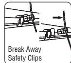
The break away safety clips that are attached to each panel and cord on the reverse of the blind will break away from the front of the clip if any reasonable weight is placed on the cord on the back of the blind. Our clips will break away leaving one side of the clip on the tape and the other on the cord.
