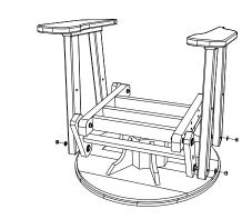
1.Attach (D) Armrest Assemblies to (A) Swivel Base using 2 Nuts & 4 Washers per side, Be sure to match all numbers & or letters.
