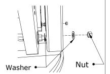
3. Slide Seat & Back between Armrests & attach to Armrests using
