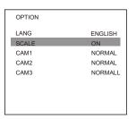
Press  $\Delta \odot / \nabla \odot$  to select ON/OFF.Scale refers to the reversing distance indicator displayed on the monitor.
