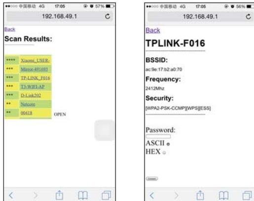
4. Dongle is able to access Internet through AP. AP's SSID and dongle's IP address that are dispatched from AP (“Device IP1”) will be shown on the screen. The mobile phone/laptop/tablet that is connected to dongle allows to access the Internet because of AP bridge function of dongle. Then long press “M” button to upgrade within 30 seconds.
