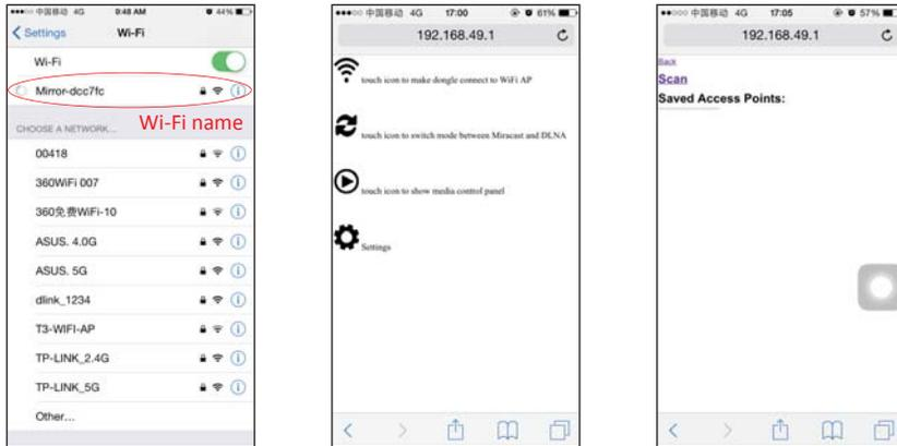
3. Tap “Scan” and follow the instructions to connect to Wi-Fi AP which allows to access Internet through WAN. Please note that when the connection between dongle and AP is established, the connection between dongle and mobile phone/laptop/tablet may be disconnected. The reason is that the connection channel between dongle and mobile phone is different from the channel between dongle and AP. In this case, mobile phone /laptop/tablet should be connected to dongle by using soft AP again.
