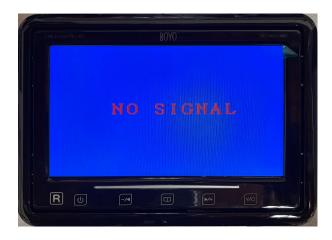
When powered on without any cameras connected, it will show a blue screen with 'NO SIGNAL'. The monitor operations require pressing of the touch buttons.
