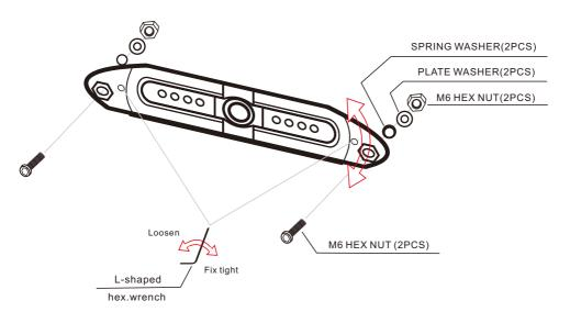
Loosen the allen screws to adjust the camera angle up and down. Then, lock it in place.
